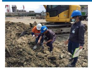
RemScan is used to sort clean soil from contaminated, thereby minimising the amount of soil to remediate.
