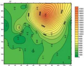
RemScan is used to measure the concentration of oil on the surface of the soil enabling the user to quickly delineate the contaminated area. Depth profiles can be measured by taking a drill core, laying the core out and using RemScan to directly measure the hydrocarbon concentration at various points (depths) along the core.
