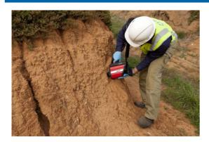
While excavation work is being performed, RemScan can measure the remaining soil to check whether all of the contaminated soil has been removed and whether the remaining soil is clean. Once all contaminated soil has been removed, samples can be sent to the laboratory for final auditing and statutory signoff.
