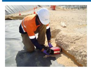
RemScan is used to monitor the soil after remediation to ensure that it complies with site requirements. For bioremediation processes, RemScan can monitor the decrease in the concentration of the contamination over time to determine the end point. Once the soil is "clean", it can be removed from the bioremediation pad, thereby increasing the utilisation and throughput of the bioremediation facility.
