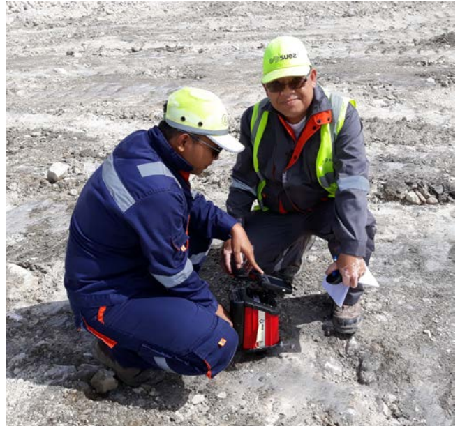
RemScan being used in-situ
