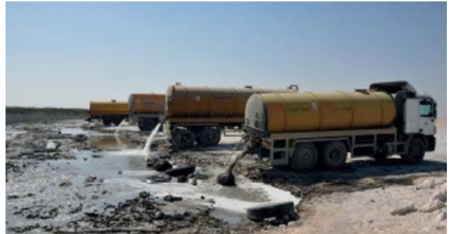
Tankers discharging wastewater into lagoons
