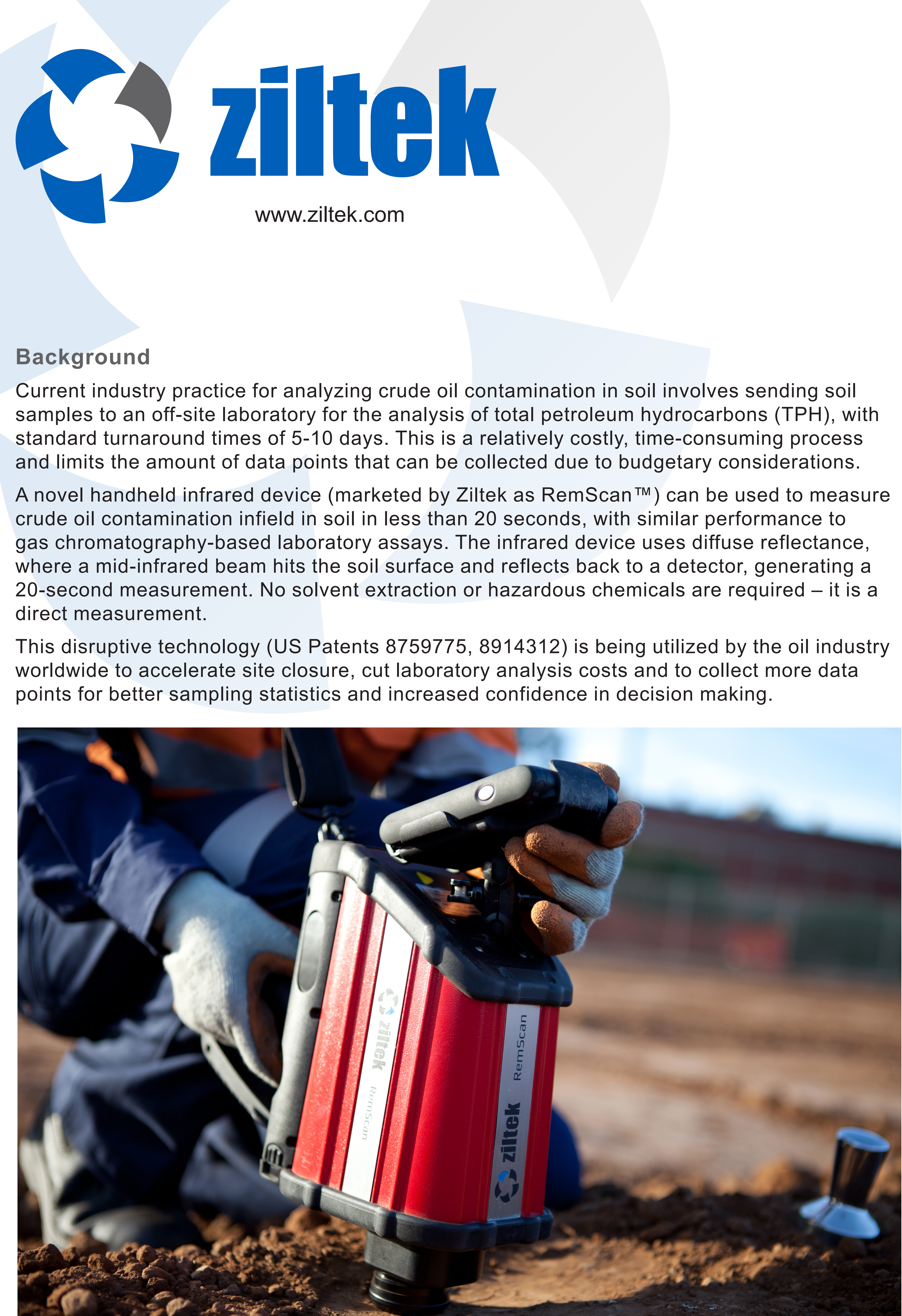
Figure 1: RemScan™; a handheld infrared device for rapid measurement of TPH in soil.
