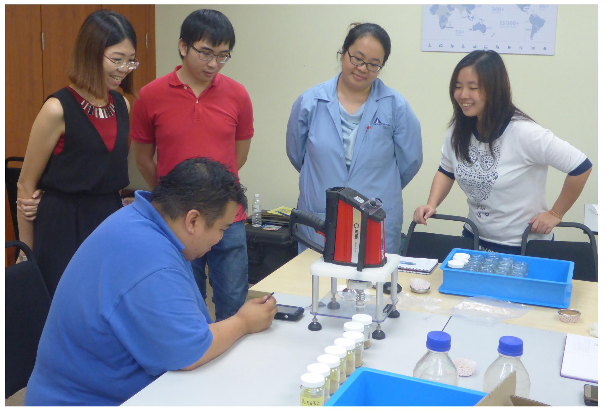
Figure 1: Scanning calibration samples using RemScan.
