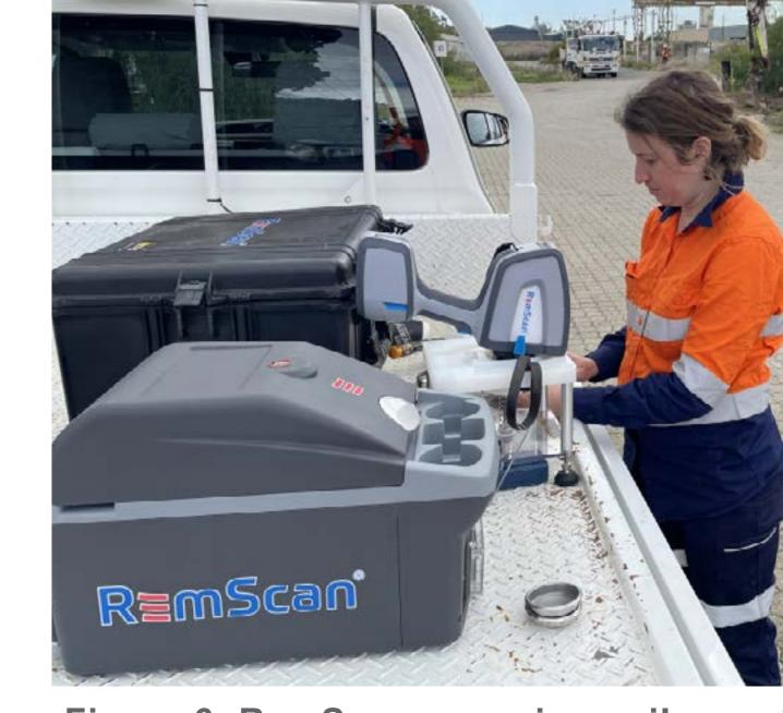
Figure 6: RemScan scanning soils ex-situ
