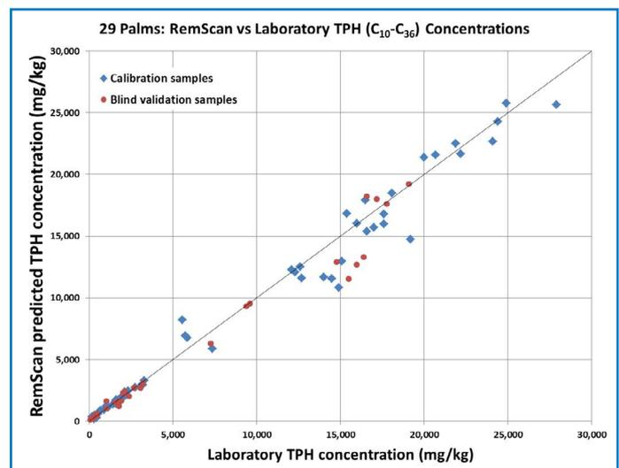
Figure 2: RemScan predictions versus laboratory assay values for calibration samples (blue) and blind validation samples (red) for the 29 Palms test site
